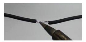
Remove the soldering iron and wait a few seconds to let the soldered connection cool and harden. Use heat shrink to cover the connection.
