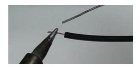
Hold the two tinned wires on top of each other and touch the soldering iron to both wires. This process should melt the solder and coat both wires evenly.
