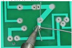
**Step 4: Snip The Leads** – Remove the soldering iron and let the solder cool down naturally. Don't blow on
