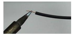
Keep the iron in place and touch the solder to the wire until it's fully coated. Repeat this process on the other wire.
