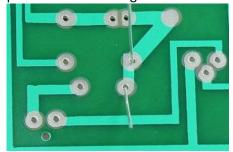
**Step 2: Heat The Joint** — Turn your soldering iron on and if it has an adjustable heat control, set it to 400'C. At this point, touch the tip of the iron to the copper pad and the resistor lead at the same time. You need to hold the soldering iron in place for 3-4 seconds in order to heat the pad and the lead.
