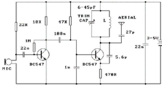
The circuit consists of two separate stages. The first is an audio pre-amplifier and the second is a 90MHz oscillator.
